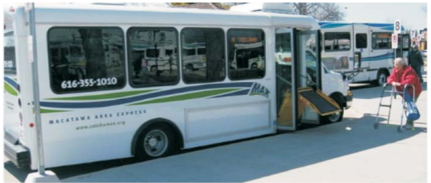
The lift lowers for a MAX customer. MAX says the Spirit of Mobility allows passengers greater control over their transit experience.
