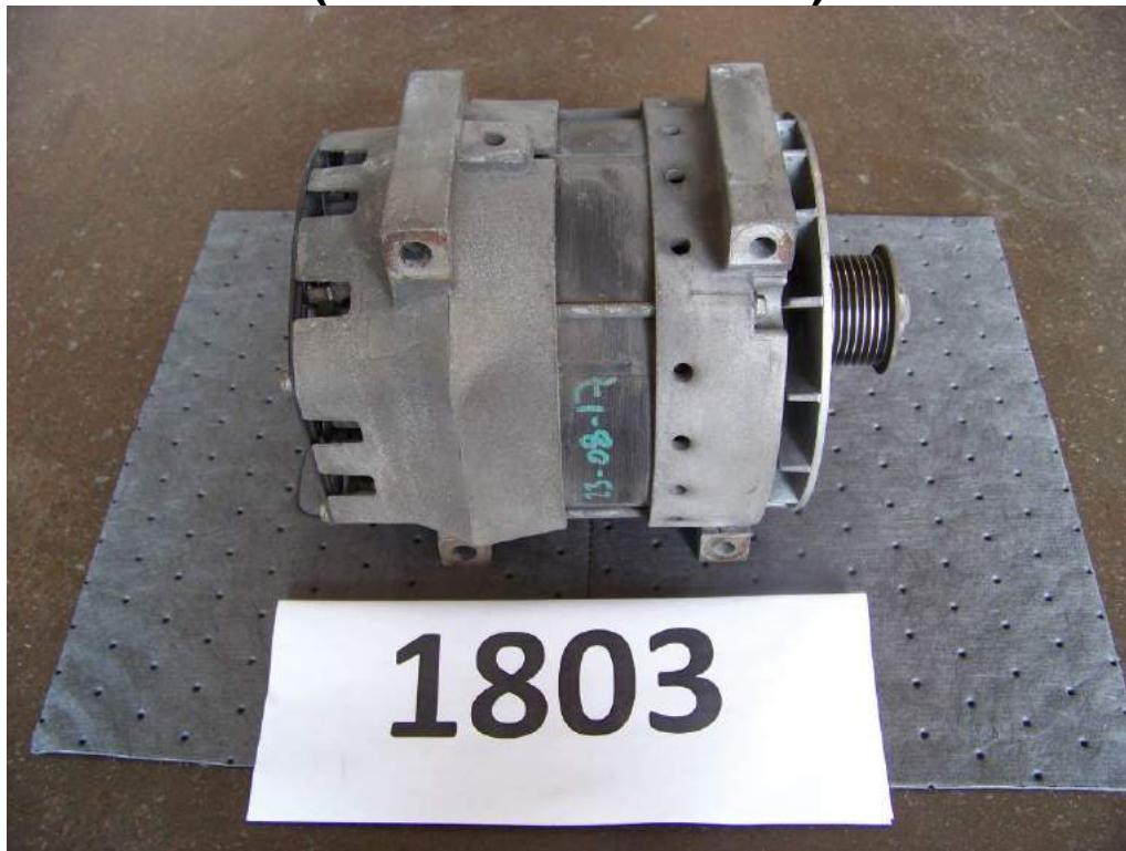
ALTERNATOR REMOVAL AND REPLACEMENT (0.5 LABOR HOURS)
