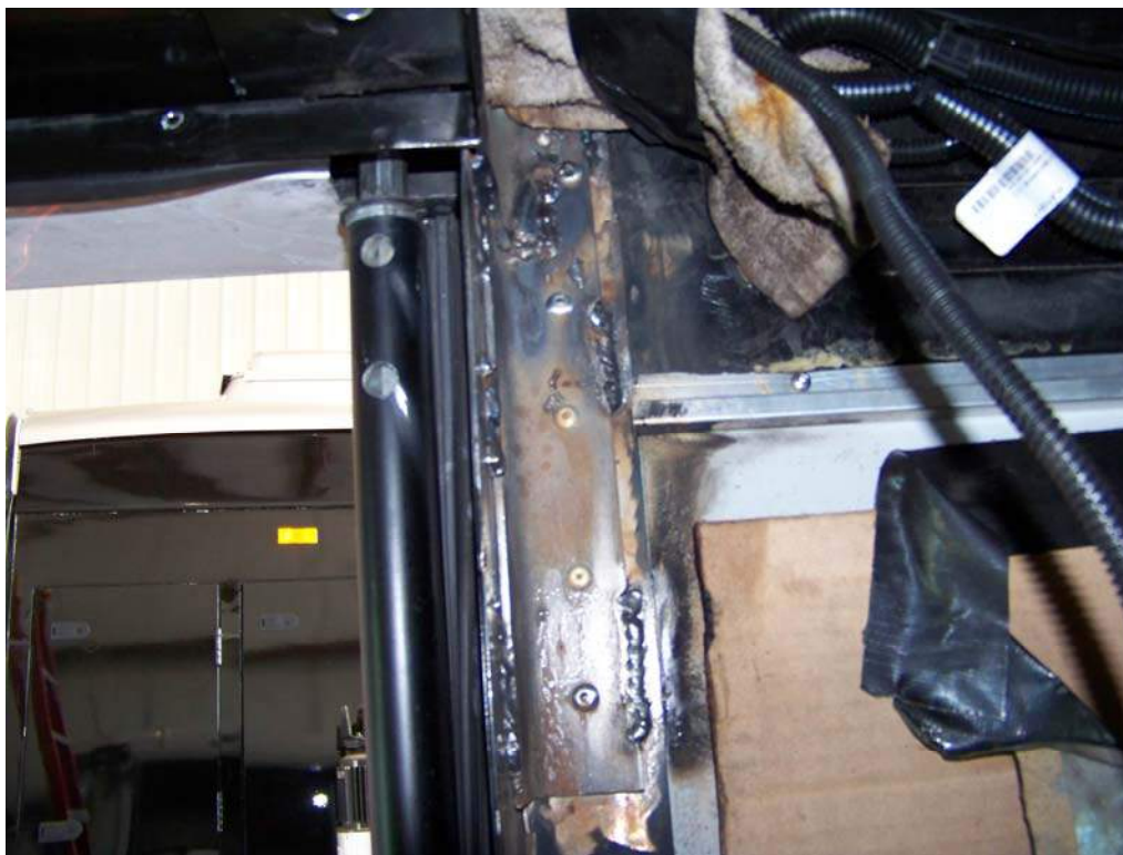
DOOR FRAMEWORK REPAIRS (5,724 TEST MILES)
