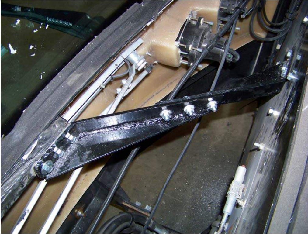
LOWER WINDSHIELD SUPPORT ADDED AND REPAIRED (1,254 TEST MILES)
