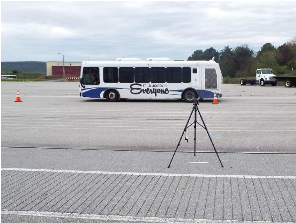
TEST BUS UNDERGOING EXTERIOR NOISE TESTING
