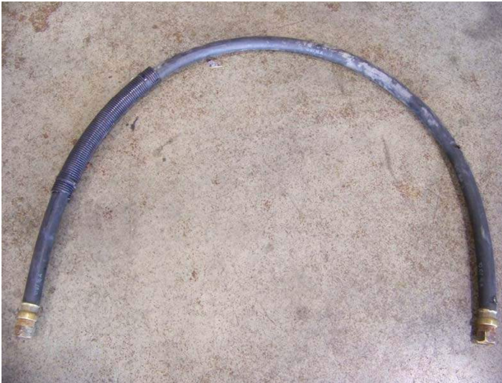
FRONT BRAKE AIR HOSE LEAK DUE TO WHEEL CONTACT (7,931 TEST MILES)
