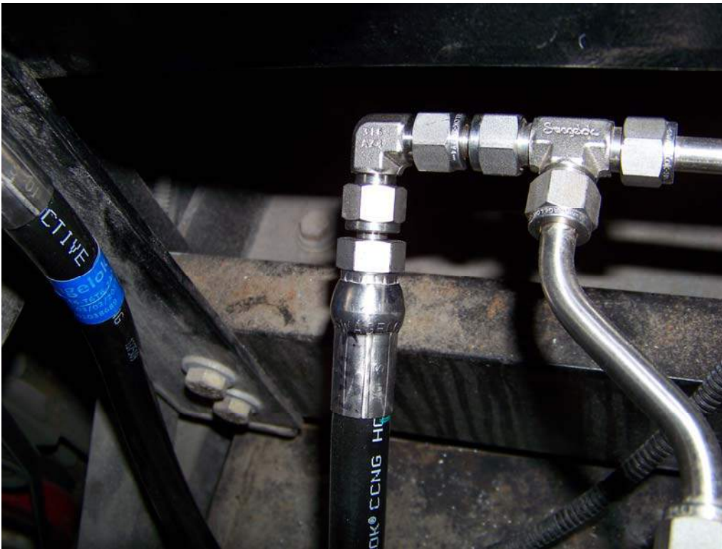
FLEX CNG LINE INSTALLED BETWEEN TANKS AND SUPPLY (1,487 TEST MILES)
