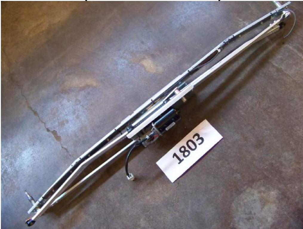
WIPER MOTOR REMOVAL AND REPLACEMENT (0.5 LABOR HOURS)
