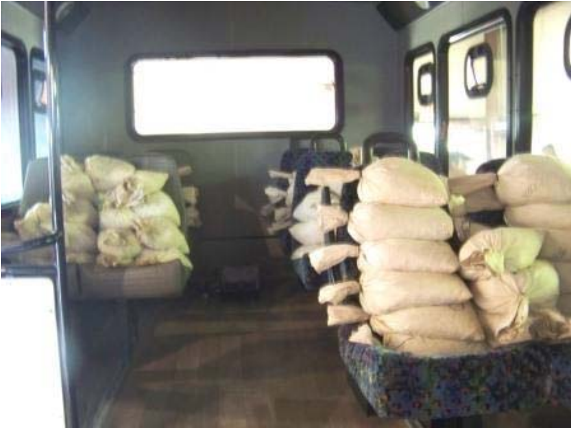
BUS LOADED TO 2.5 TIMES GVL (4,125 LBS)
