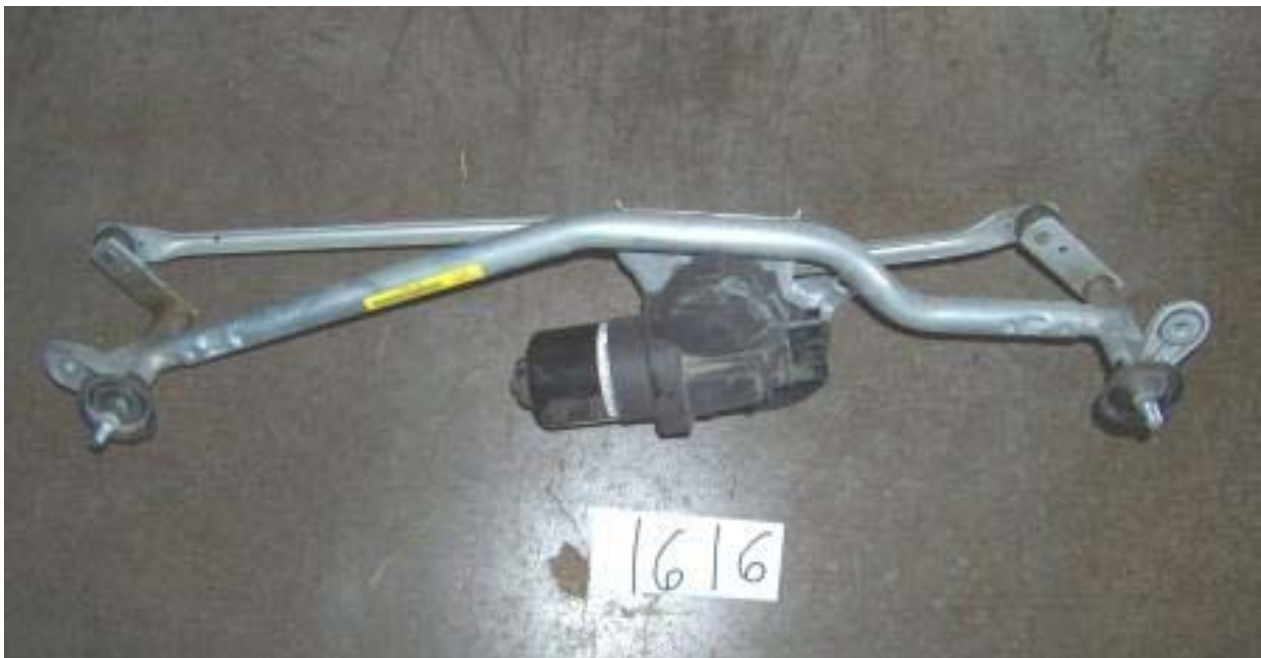
WIPER MOTOR REMOVAL AND REPLACEMENT (1.0 MAN HOURS)
