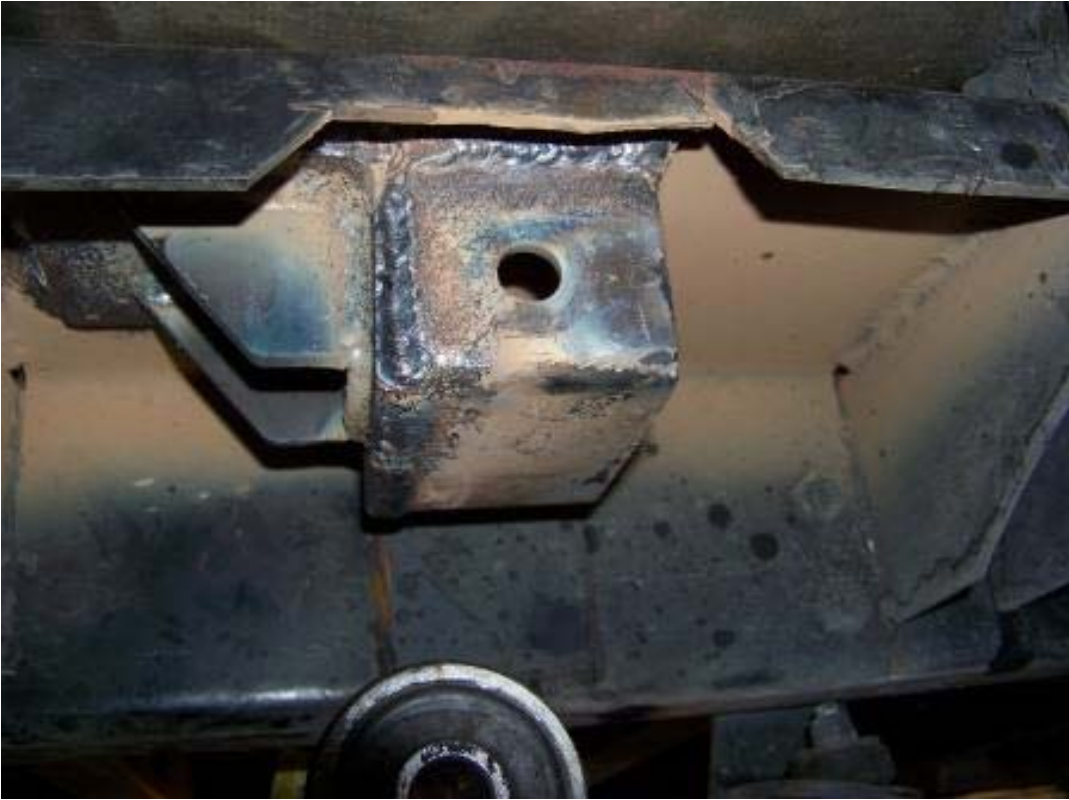
REPAIRED REAR SPRING HANGERS (1,882 TEST MILES)
