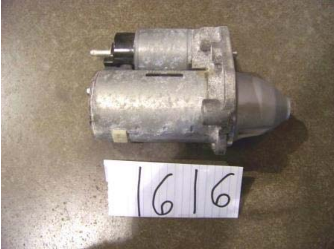
STARTER REMOVAL AND REPLACEMENT (1.25 MAN HOURS)
