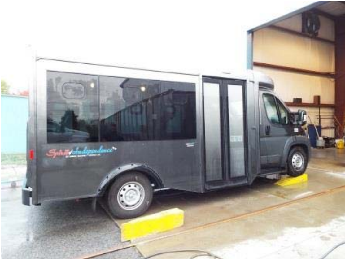
RIGHT FRONT WHEEL SIX INCHES HIGHER
