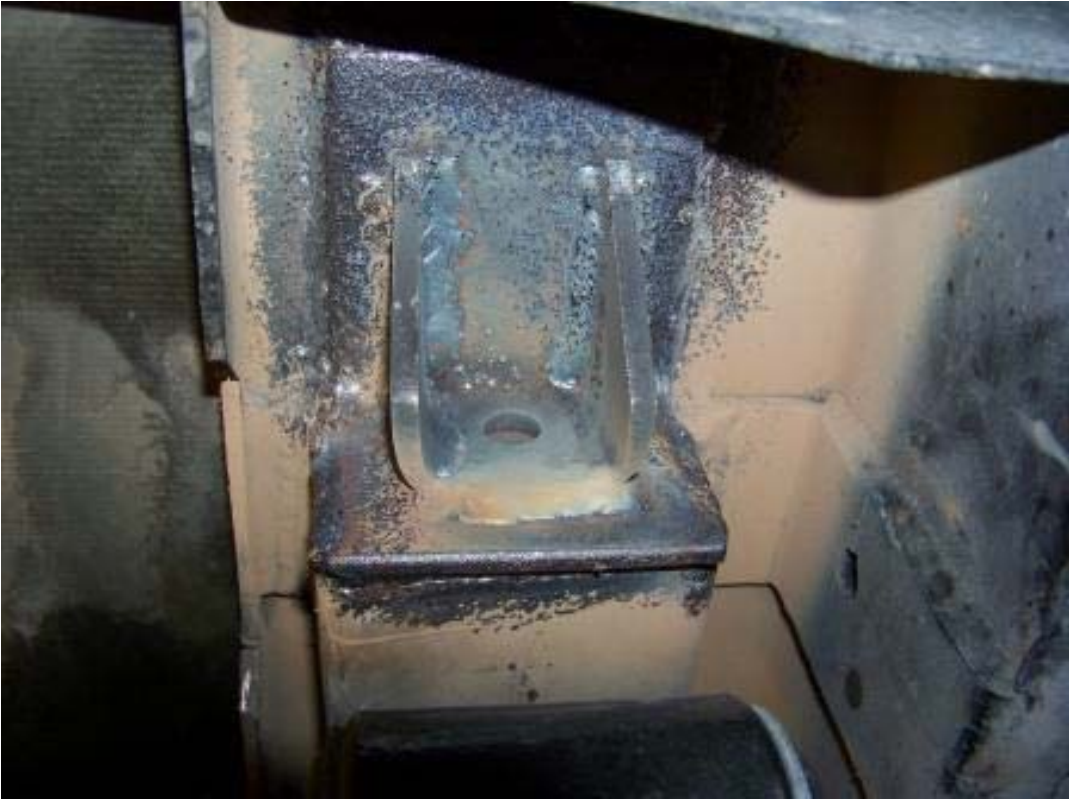
REPAIRED REAR SPRING HANGERS (1,882 TEST MILES)
