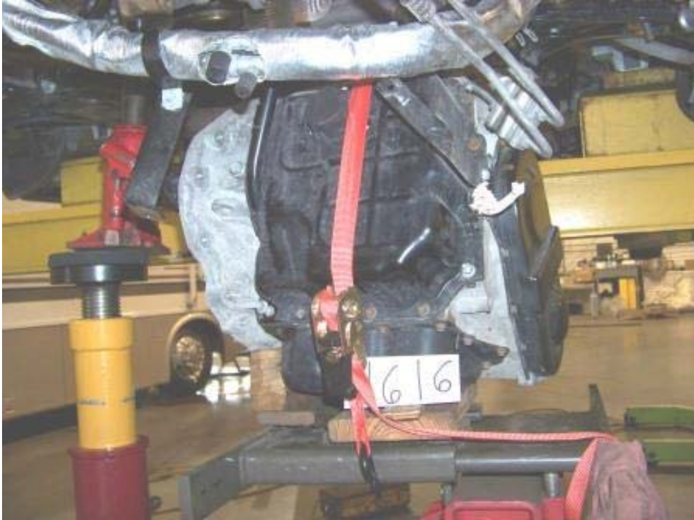
TRANSMISSION REMOVAL AND REPLACEMENT (9.5 MAN HOURS)
