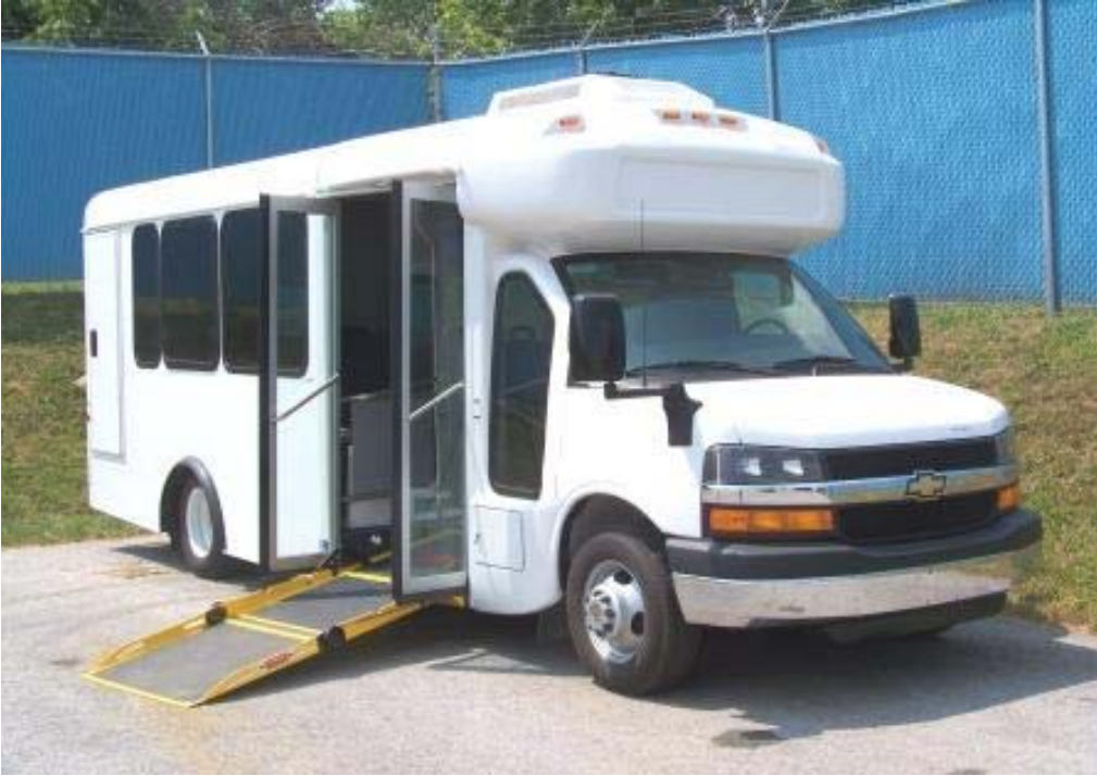
ARBOC MOBILITY, LLC. MODEL 2010 CNG HYBRID-SOM236 EQUIPPED WITH A BRAUN HANDICAP RAMP
