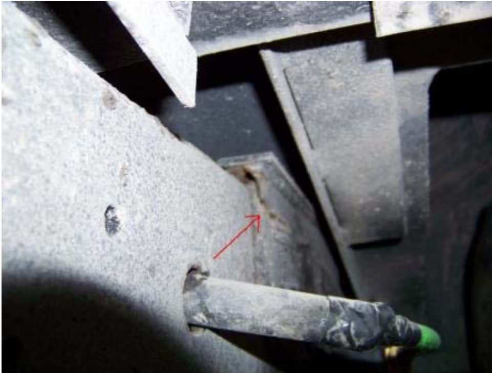
FRAME CRACK AT ABOVE REAR AXLE (3,204 TEST MILES)
