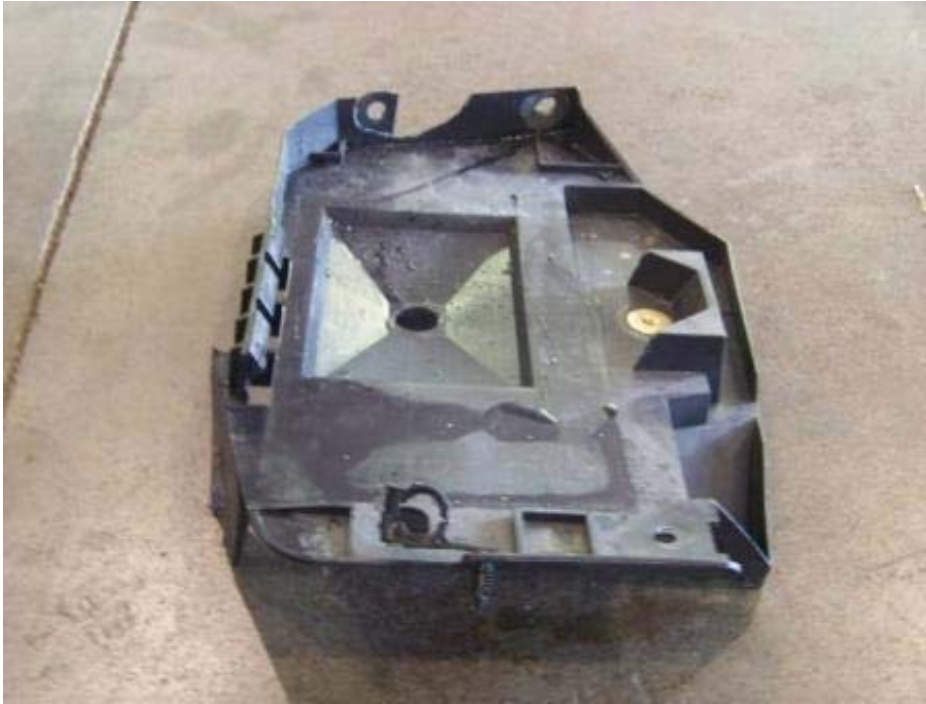
FAILED BATTERY TRAY (3,204 TEST MILES)
