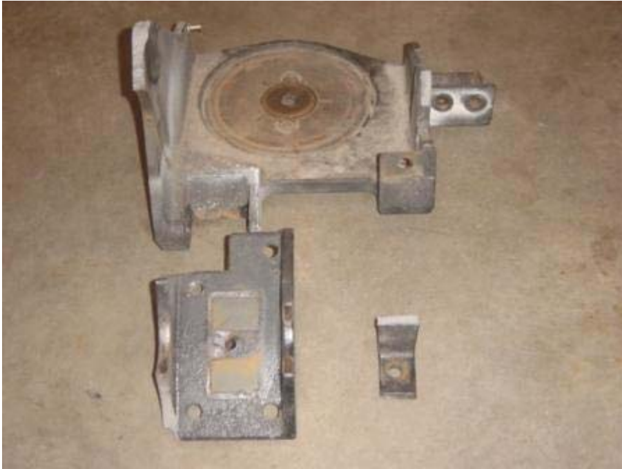
BROKEN RIGHT REAR AIR BAG PEDESTAL (2,202 TEST MILES)
