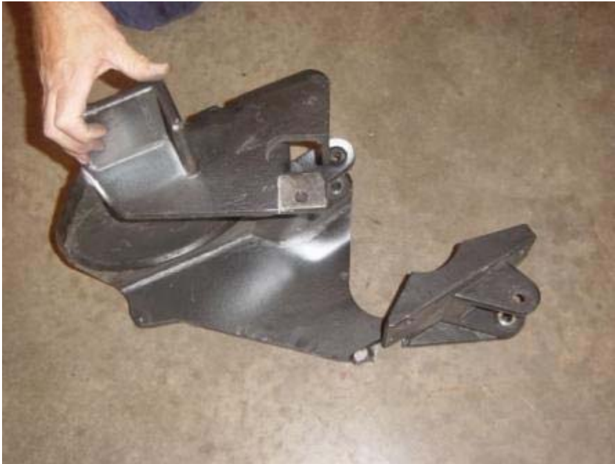
BROKEN RIGHT REAR AIR BAG PEDESTAL (2,661 TEST MILES)
