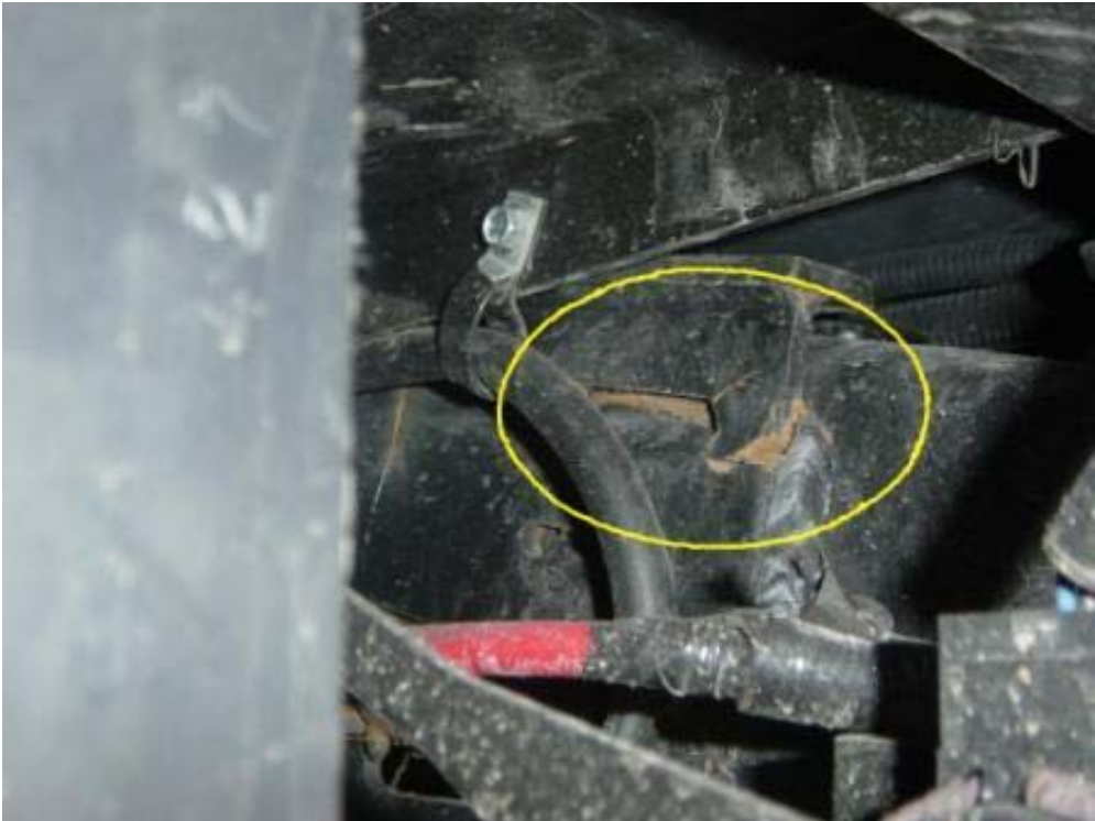
CRACKED FRAME RAIL (630 TEST MILES)
