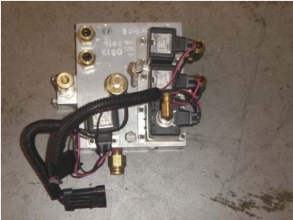
FAILED AIR CONTROL BOARD (1,214 TEST MILES)
