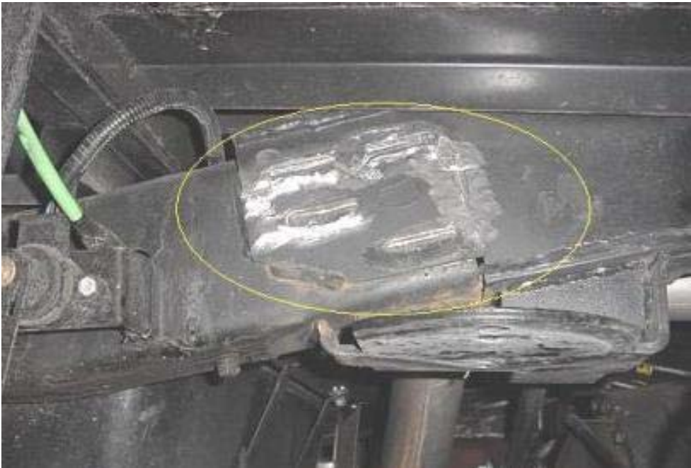
CRACKED FRAME RAIL (630 TEST MILES)
