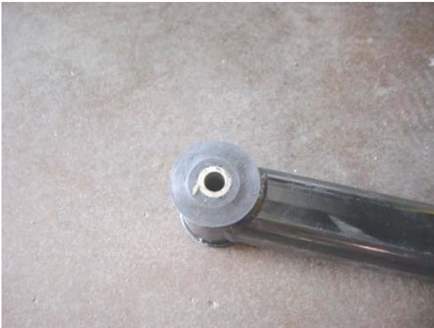
TRAILING ARMS INSTALLED WITH NEW TYPE BUSHING (1,253 TEST MILES)
