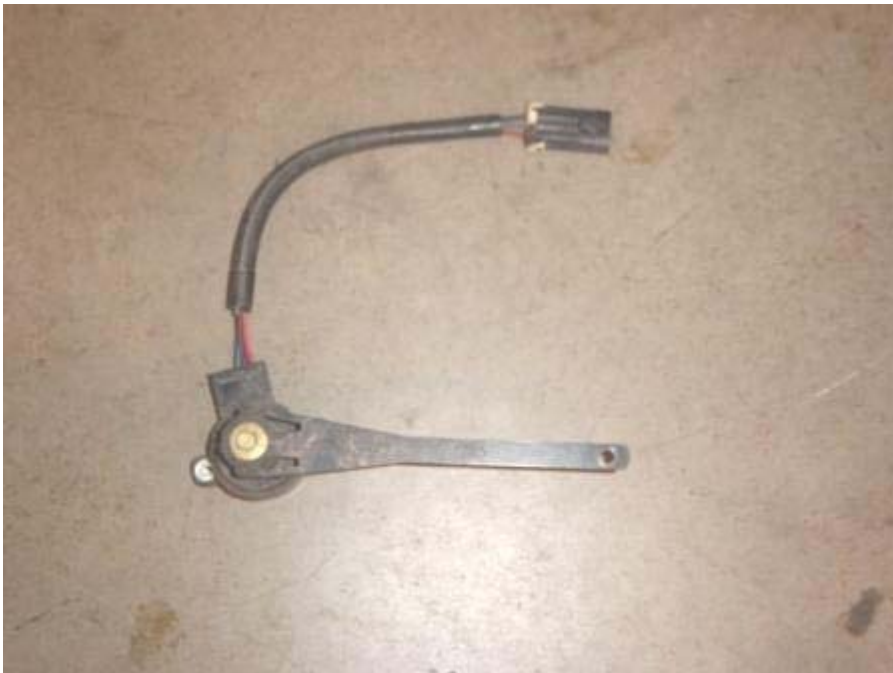
FAILED LEVELING VALVE (2,659 TEST MILES)
