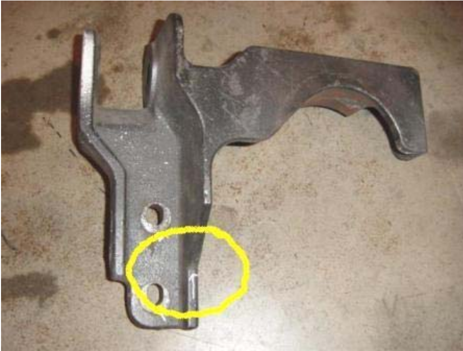
CRACKED REAR LATERAL BAR MOUNT (5,071 TEST MILES)
