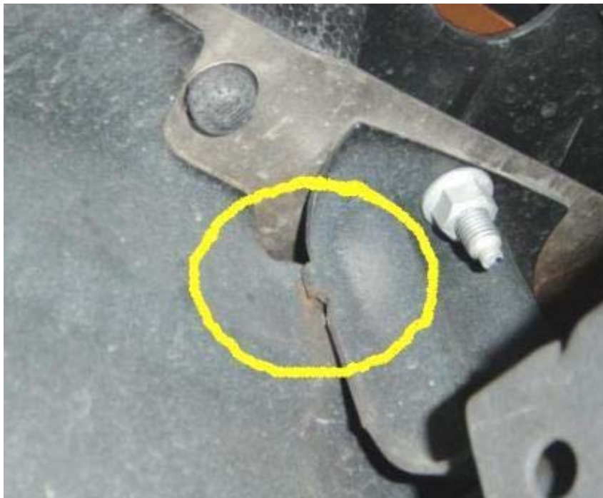
BROKEN FRONT BUMPER BRACKET (5,515 TEST MILES)
