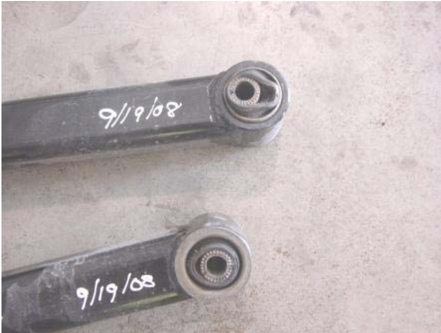
WORN BUSHINGS IN LOWER TRAILING ARMS (1,253 TEST MILES)
