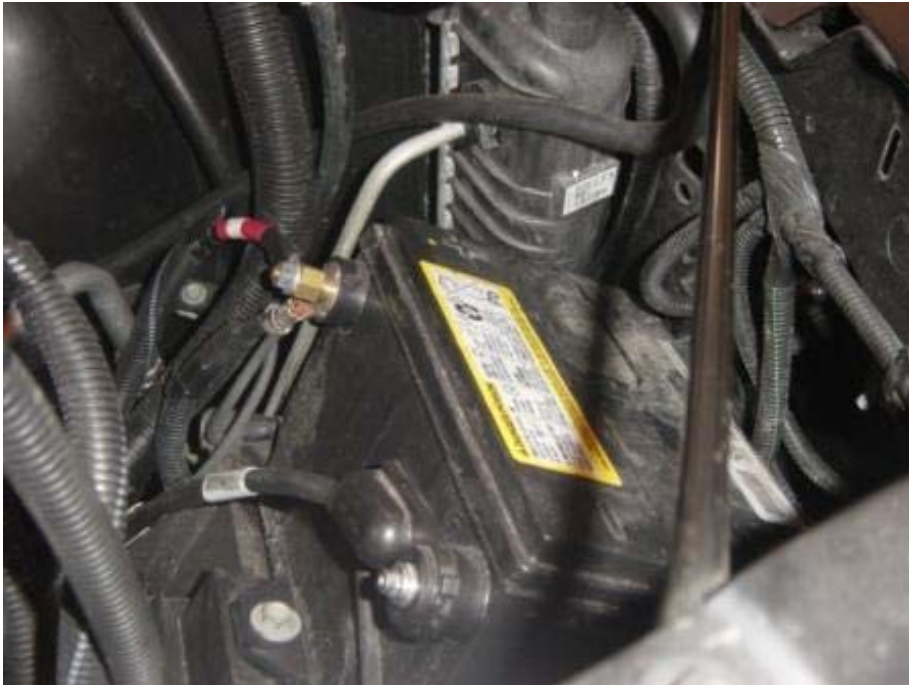
LOOSE BATTERY AND BATTERY BOX (2,146 TEST MILES)
