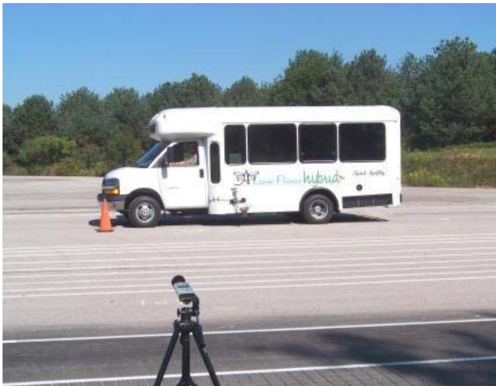
TEST BUS UNDERGOING EXTERIOR NOISE TESTING
