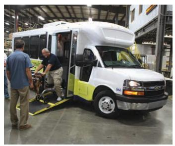
Low-floor bus manufacturers like ARBOC Specialty Vehicles exceed many of ADA's current guidelines, including ramp entry with lesser degree slopes of 1:5 and 1:6
