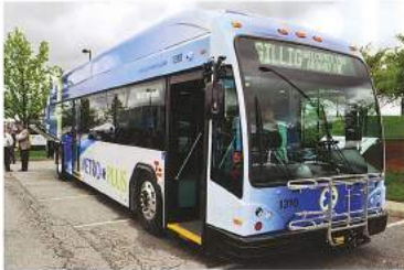
▲ Gillig's new BRTPlus bus was used for shuttling show attendees before it heads to Cincinnati's SORTA. It features a unitized stainless steel chassis with a unique side-impact barrier to add strength and corrosion resistance as well as protect passengers in the event of a collision.
