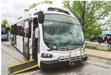
▲ Proterra's EcoRide BE35 is the first zero-emission full-size bus to pass Altoona-testing and was proven to have both the highest fuel economy (22 mpg average) and lowest noise (57 dBA or 10 times lower) of any full-size passenger bus ever tested.
