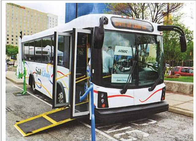
▲ Arboc's Spirit of Liberty features a lightweight "Bolt-N-Bond" hybrid composite construction that is 30% lighter, which contributes to a 6% gain in fuel economy, and is designed to address and exceed 2014 to 2018 economy standards.
