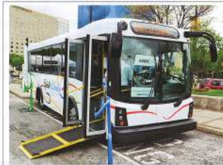
▲ Arboc's Spirit of Liberty features a lightweight "Bolt-N-Bond" hybrid composite construction that is 30% lighter, which contributes to a 6% gain in fuel economy, and is designed to address and exceed 2014 to 2018 economy standards.
