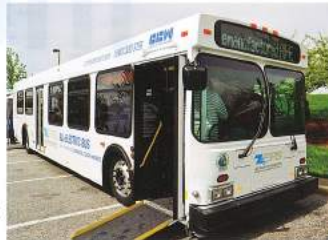
▲ MCI's team was on hand to showcase Denver RTD's new Commuter Coaches, which are equipped with a wheelchair lift and an ACTIA multiplex system as well as an ergonomic driver dash and the latest clean-diesel engine technology for near-zero emissions.
