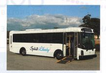
Next, the Spirit of Freedom utilizes only General Motors standard suspension to create a low-floor, ADA compliant bus capable of 1:6 ramp angle; all with an exceptional ultra-low price point. With the spacious 41" entry opening and low step height, makes this an ideal bus for airport, hotel, and resort shuttles, as well as transit agencies.
