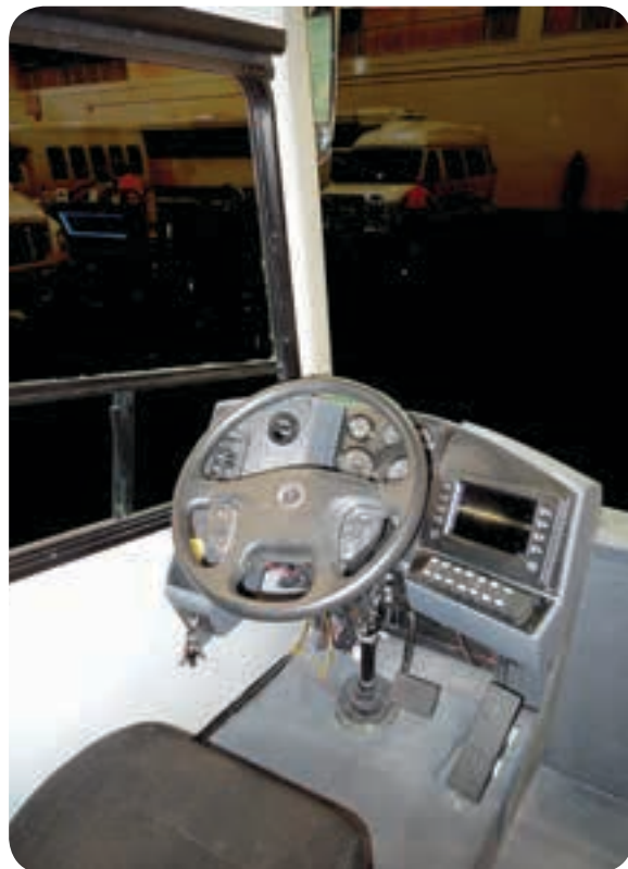
The asymmetric windshield minimizes blindspot and blockage from the column from the driver's seat.
