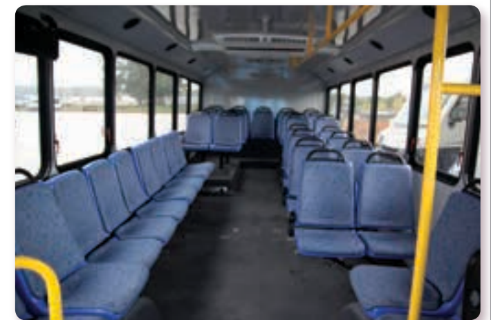
Open low-floor passenger area with no steps, oversize wheelchair positions and weight-reducing technology address key operator concerns.
