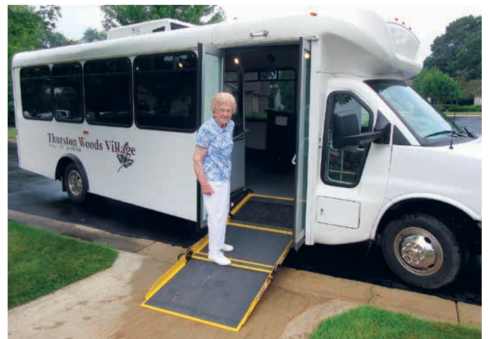
A ramp allows everyone to use the same entrance door, which creates a sense of equality among all passengers.
