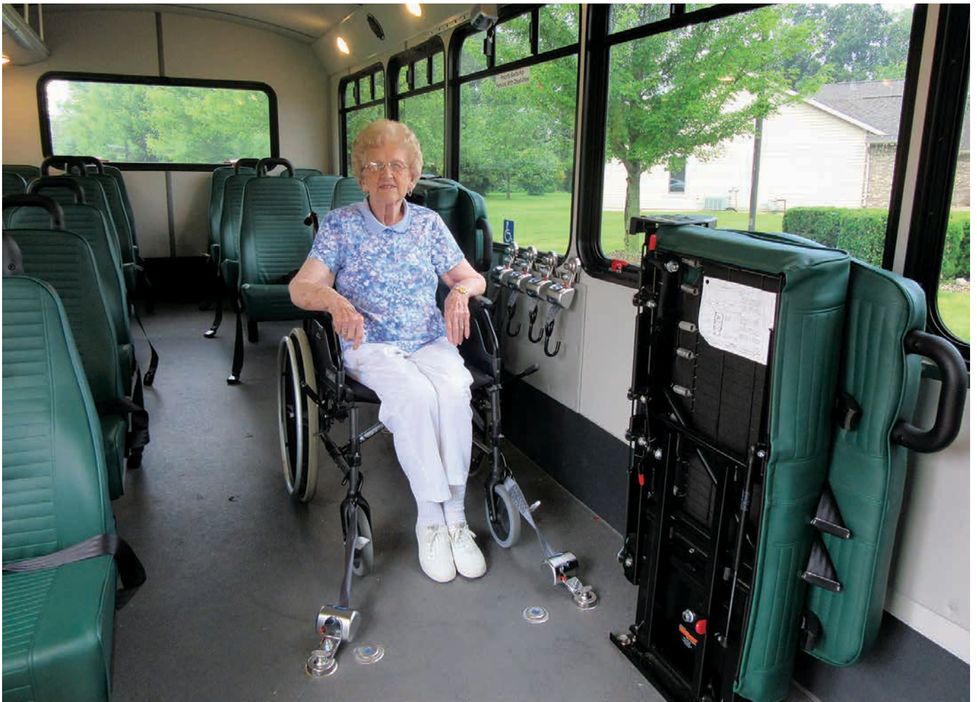
Complete with the tiedown process, loading a wheelchair-using passenger onto a low-floor bus takes approximately two minutes.
