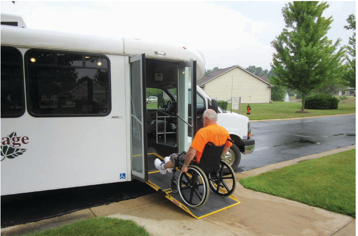
A ramp allows passengers with wheelchairs to board a bus without assistance.
